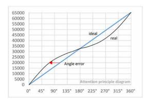
The singleturn repeat accuracy describes the tolerance of the position of the measured and transmitted position value to a reference position or in reverse mode. This means that if the same position or a previously approached reference point is approached several times, the measured and transmitted position value varies with an error in a smaller tolerance band.
